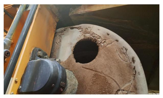
**Image 1 –** Struvite Removed in Areas Prior to HydroFLOW Installation
